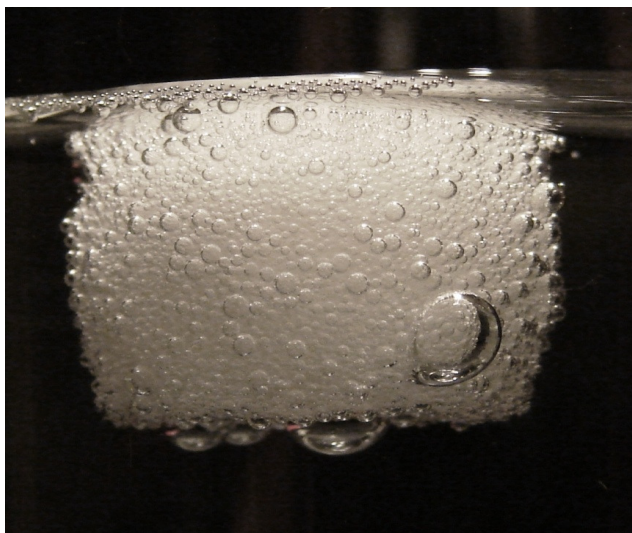
Figure 22. Bubbles entrapped in the gellified matrix after 4 h
