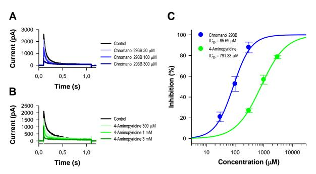
**Figure 11.** Concentration-dependent blocking effects of chromanol 293B and 4-aminopyridine on Kv1.4 currents. Panel **A** and **B** present representative current curves recorded during application of increasing concentrations of chromanol 293B and 4-aminopyridine. Panel **C** shows the dose-response curves of the reference compounds. The estimated  $IC_{50}$  values were 85.69 ± 8.38 µM (n = 4) and 791.33 ± 26.84 µM (n = 4), respectively.
