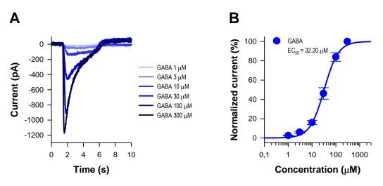
**Figure 4.** Effect of GABA on whole-cell current. Panel **A** depicted sample current curves evoked by different concentrations of GABA. Panel **B** shows the dose-response relationship of GABA. The EC<sub>50</sub> value was determined to  $32.20 \pm 1.85 \mu M$  (n = 5) by plotting the normalized peak current amplitudes against concentration.
