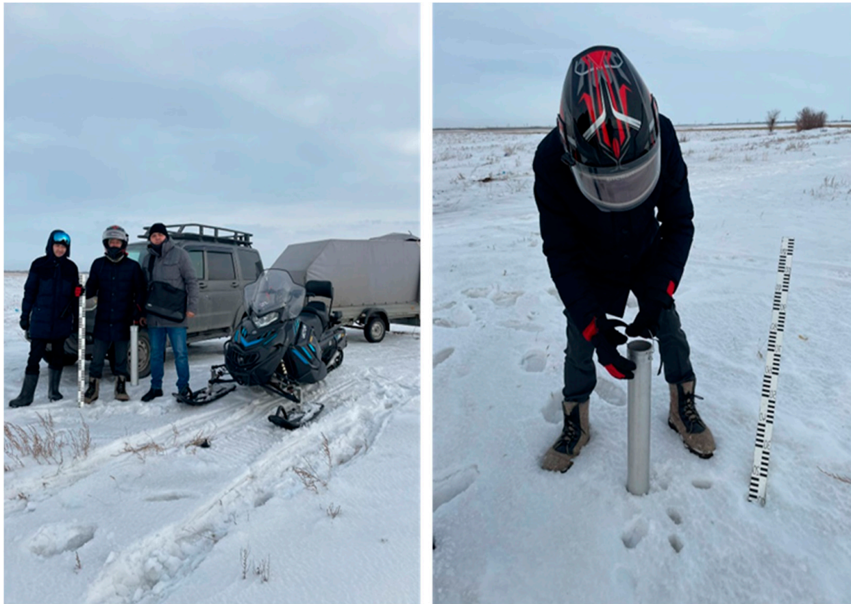
Figure A1. The process of measuring the snow height and density.
