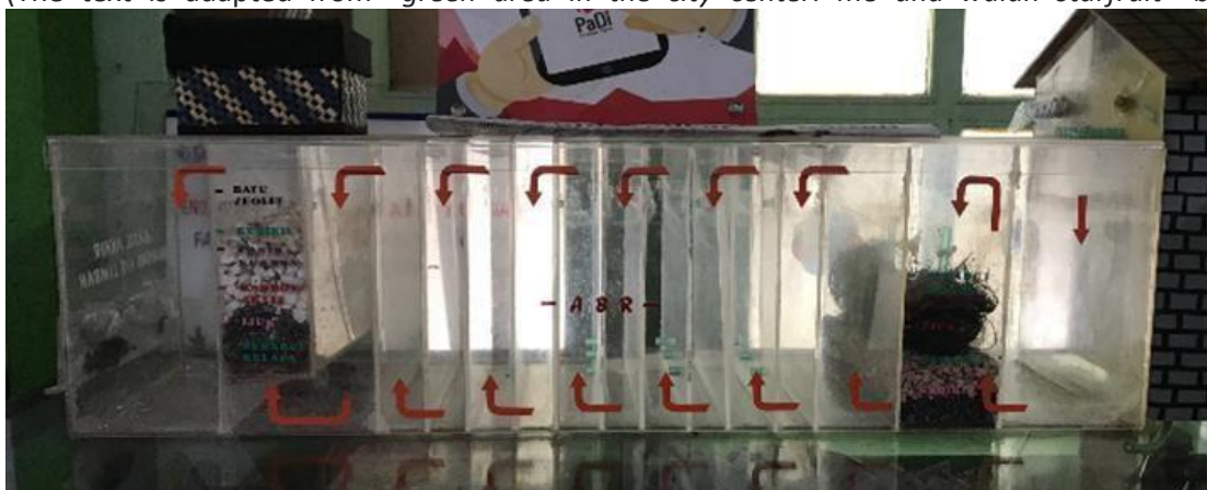
Mock-up Pandora L (Waste water recycling)
