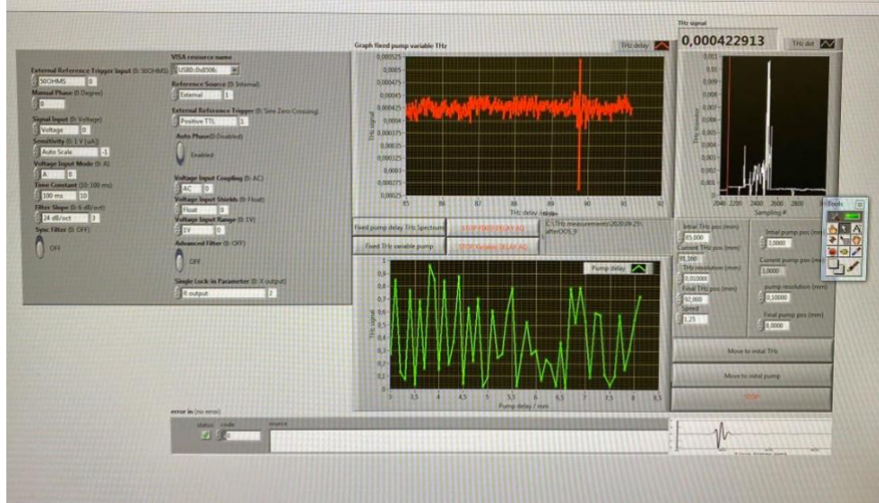
Figure 42. Front panel of the custom-built LabVIEW software used for THz time-domain measurements. Users can set the scanning range, step size, resolution, and speed, as well as configure all lock-in amplifier parameters. The red curve displays the measured THz signal as a function of the probe delay.
