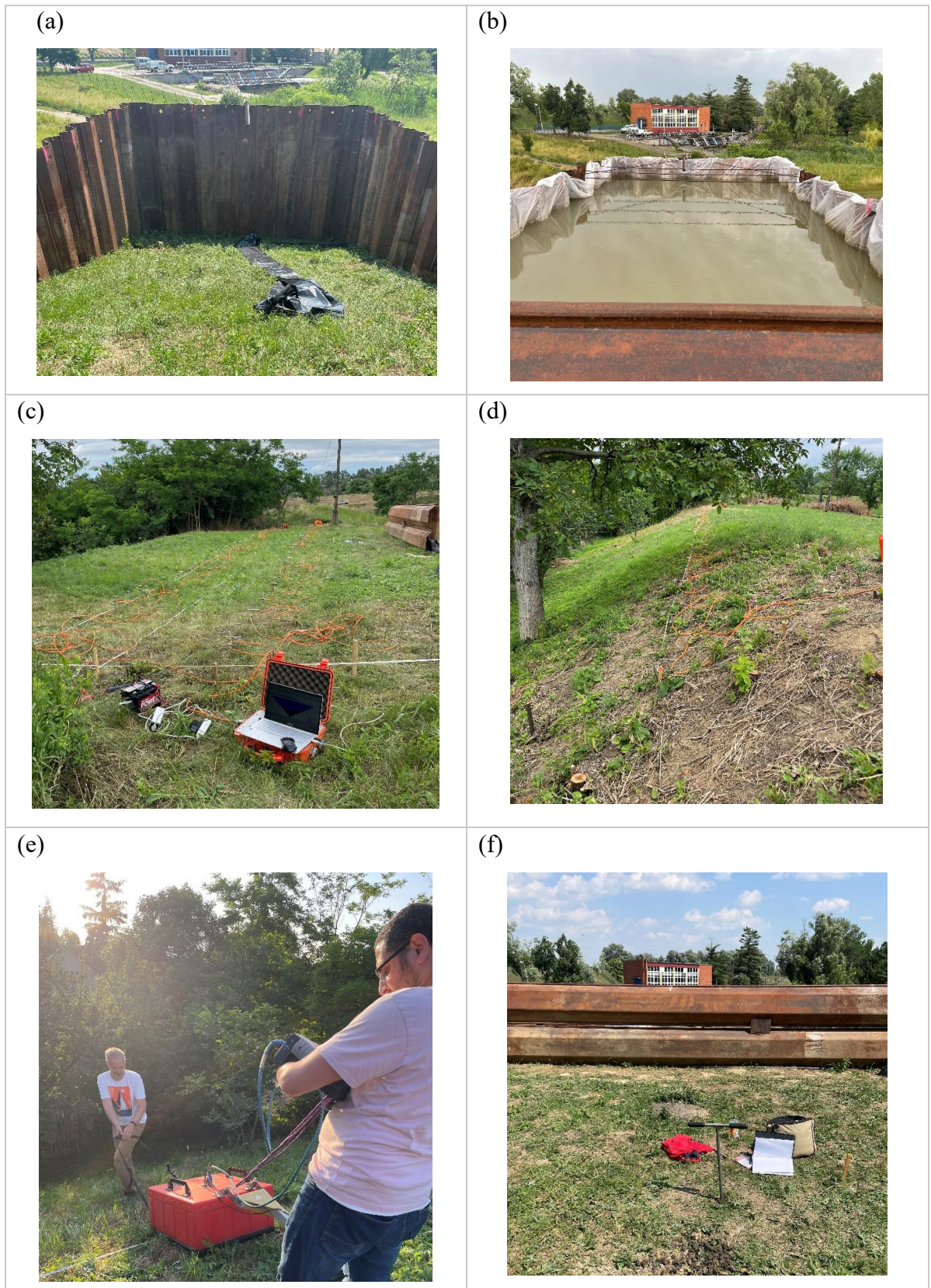
Figure 2.2 Field photos of the tank (a) before and (b) after filling with water; ERT data acquisition on the (c) levee crown and (d) protected side; (e) GPR data acquisition; and (f) borehole drilling
