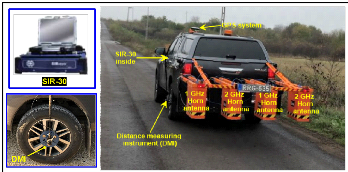
Figure 3.2 GPR data collection using SIR-30 equipped with four horn antennas.
