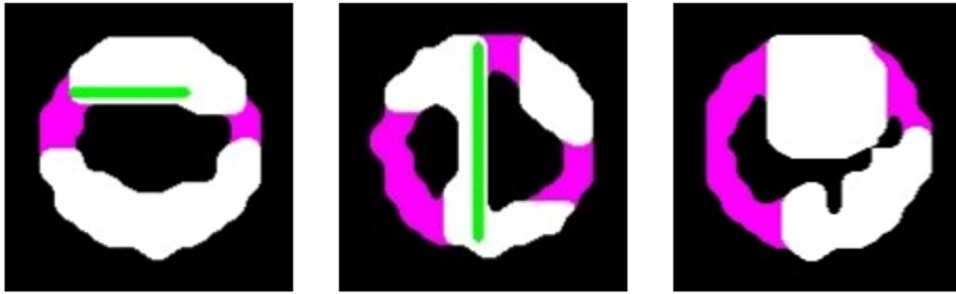
Fig. 7. Outcome of line detection marked in green. The left and middle components are identified as blink-related. White areas stem from ICA components, while purple regions originate from the bounding circle.
