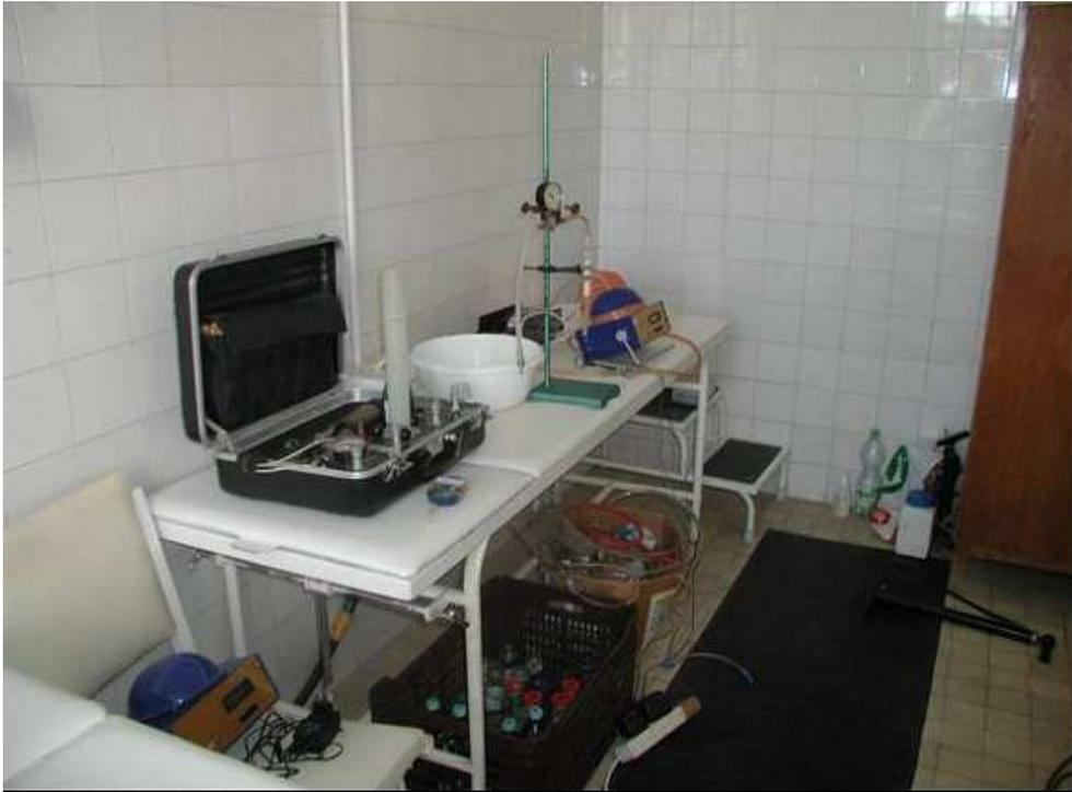
Laboratory No. 1. with diving cylinders, Lucas cells on the floor, vacuum pump by the window
