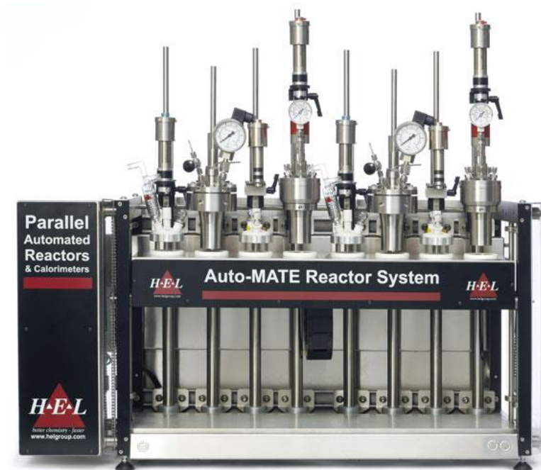
Figure 18: The Auto-MATE Reactor system by HEL.
