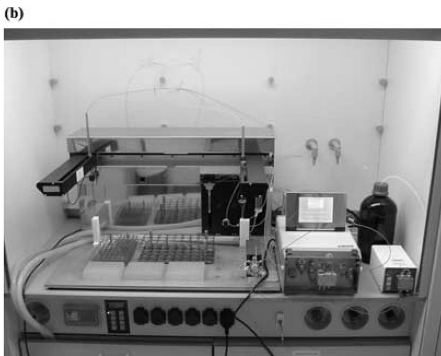
Figure 21: A continuous-flow reactor set-up for high throughput hydrogenation (a) scheme (b) photograph of set-up.
