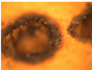
Fig. 1. Nd:YAG laser treated original tablet.
