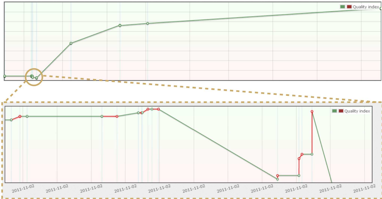
Figure 2: Maintainability of System A over the refactoring period and a selected subperiod where we highlighted in red the changes in maintainability caused by refactoring commits
