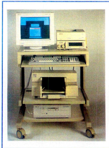
Figure 3-1 The Sonicaid Meridian 800 cardiotocograph
