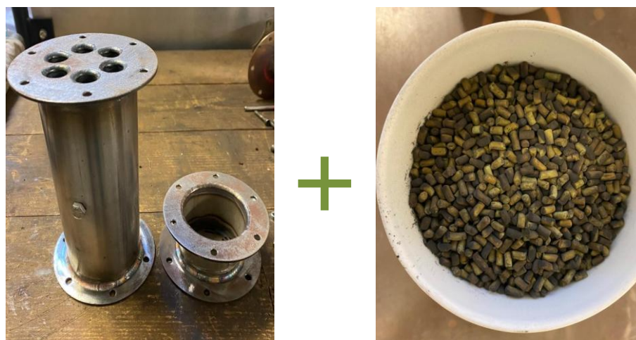
Figure 36. The utilized samples in the combined effort project including 1. The pelletized \text{Al}_2\text{O}_3 support, 2. Reactor C, and 3. The 5wt. % Co + 0.1wt. % Pd combination loading.
