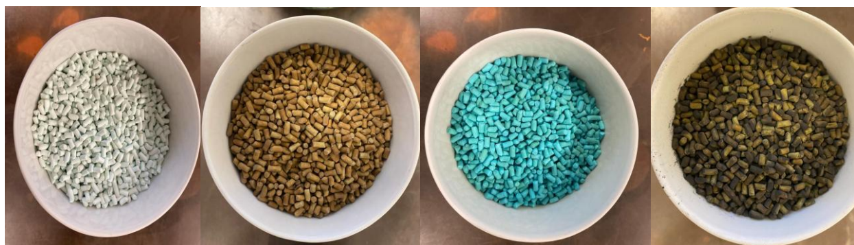
Figure 32. Pictures of the prepared catalysts where a. shows Aluminum Oxide support without loadings, b. shows a Ni/Pd sample, c. shows a Co/Pd sample, and d. shows a Cu/Pd sample.
