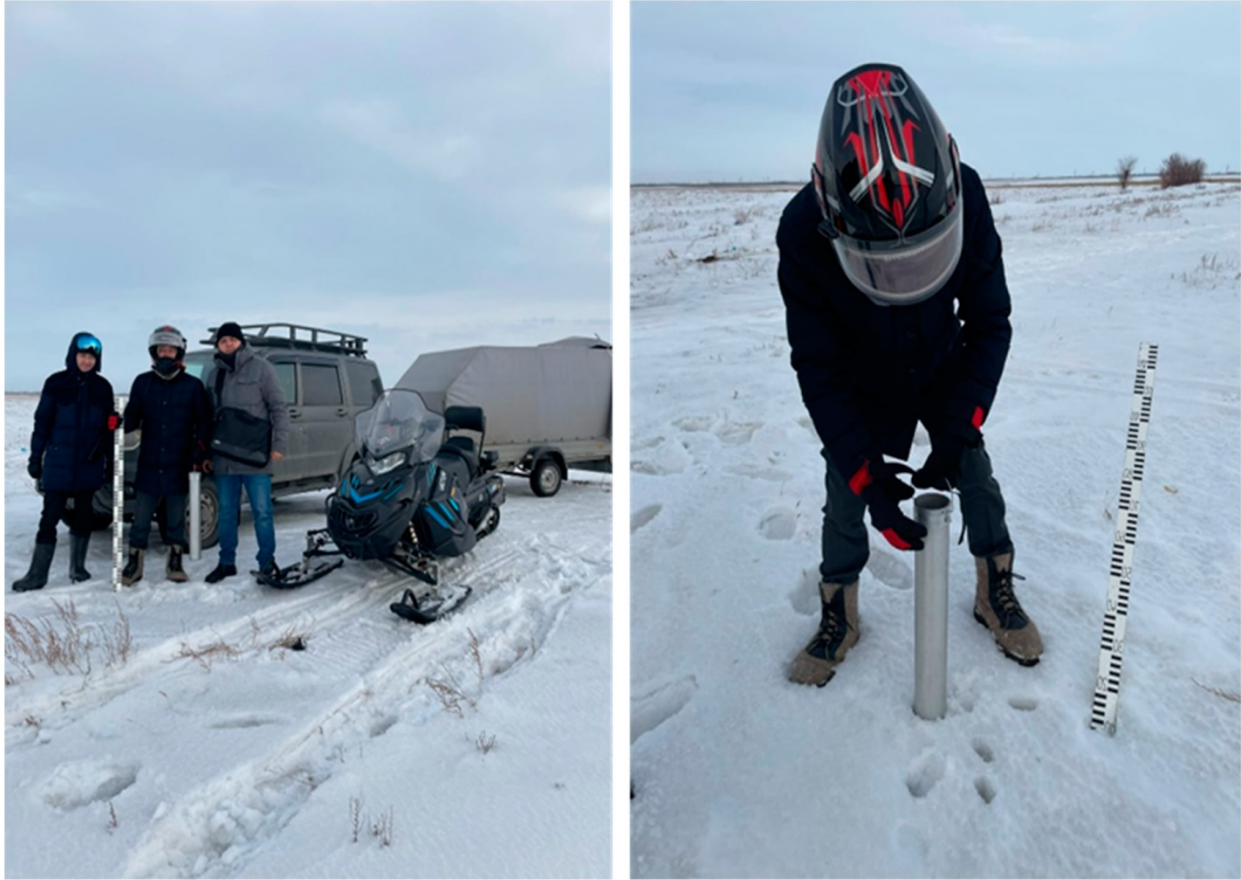
Figure B1. The process of measuring the snow height and density.
