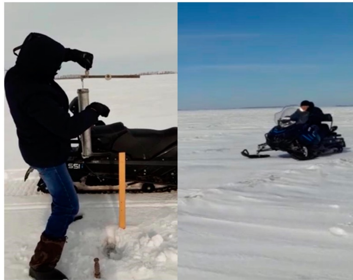
Figure 3.3. Process of measuring the snow height and density
