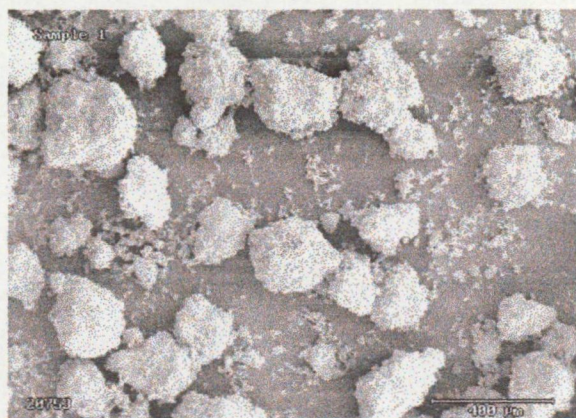
Fig. 2. Crystal agglomerates of developed MASP.
