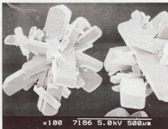
Fig. 4. Crystals of developed ASA.
