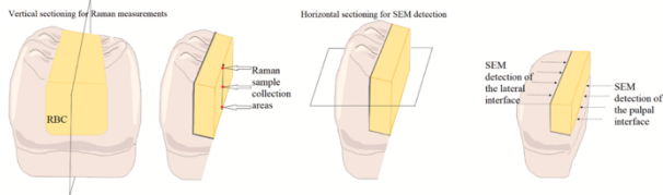
Figure 3. Schematic figure of sample preparation for micro-Raman and scanning electron microscopy (SEM) measurements. The resin-based composite (RBC) fills the cavity which has exactly the same width (2.5mm) and depth (5mm) occluso-proximally. Mesio-distal vertical sectioning provided the sample for the micro-Raman measurements at three different points along the occluso-
