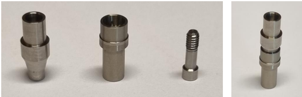
Figure 3. Pictures of a test implant and abutment used in the second-round static and dynamic tests
