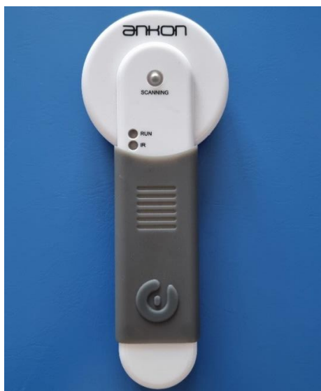
Picture 7. Manual capsule locator and activator
