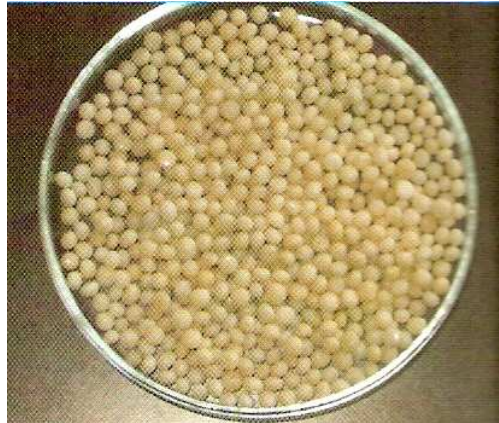
Fig. 12. A batch of Levodopa-PEG 4000 round particles prepared by dropping method
