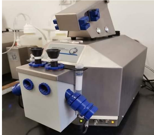
Figure 1. High-resolution respirometer (OROBOROS Oxygraph-2k (O2k). Measurements are performed by Clark-electrodes. Two chambers of the respirometer allows parallel investigations of mitochondrial functions.
