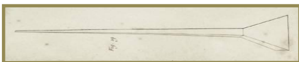
Figure 2. “Teeth-to-teeth stimulator”. A wooden rod shaped into “bone conduction hearing device” acting through “teeth-to-teeth” vibration energy transmission.
