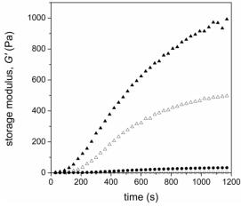
Fig. 6. Evolution of storage modulus (*G*') as a function of time at ( $\bigcirc$ ) 7% w/w and ( $\triangle$ )10% w/w polymer concentrations with (solid symbols) or without (open symbols) mucin
