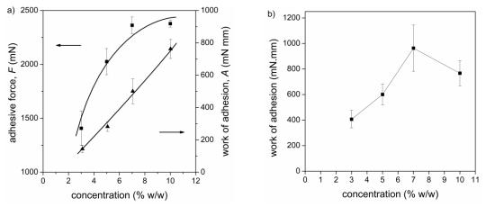
Fig. 7. (a) ( $\blacksquare$ ) Adhesive force (*F*) and (▲) work of adhesion (*A*) as functions of polymer concentration *in vitro* and (b) work of adhesion (*A*) as functions of polymer concentration *ex vivo*
