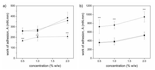
Fig. 3. Work of adhesion of ( $\bullet$ ) CLNaHA, ( $\blacksquare$ ) NaHA and ( $\blacktriangle$ ) ZnHA as a function of the concentration of the polymer a) *in vitro* (mucin) and b) *ex vivo* (porcine conjunctiva) (\*\*\*:  $p \le 0.001$ , highly significant compared with CLNaHA)
