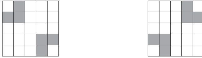
Figure 4.7: Two sets of \mathcal{Q}' with an empty row and column and the same horizontal and vertical projections
