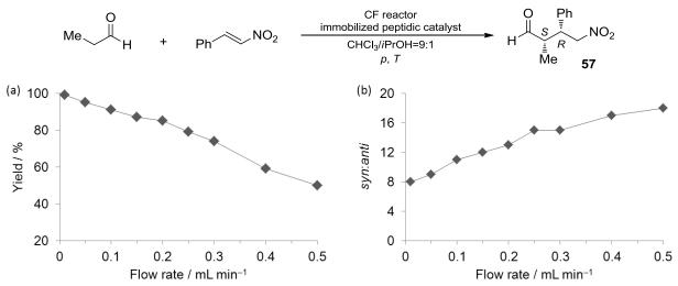
**Figure 6.** The adjustment of the flow rate in the test CF reaction between propanal and E- $\beta$ -nitrostyrene influenced not only the yield, but also the diastereoselectivity as the catalyst epimerized the  $\gamma$ -nitroaldehyde product. (Conditions: 1 equivalent of BNS (c=8 mg mL<sup>-1</sup>) and 5 equivalents of propanal, 60 bar, RT.)
