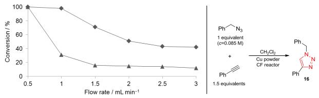
Figure 3. The flow rate dependence of the test CF CuAAC reaction between benzyl azide and phenylacetylene clearly demonstrates that the joint use of basic and acidic additives relieves the harsh reaction conditions. (▲: 100 bar, 100 °C, no additives; ♦: 100 bar, RT, 0.04 equivalents of DIEA + 0.04 equivalents of AcOH.)
