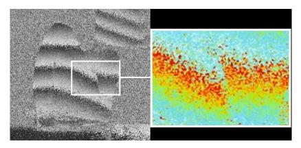
**Fig. 51.** *Screenshot 5:* SI image sample "prosthetic crown" and displacements shown in a contour colored map. The behavior for a load of 52.78 N,  $\Delta F = 30.07$  N, N ref: 82.85 N.
