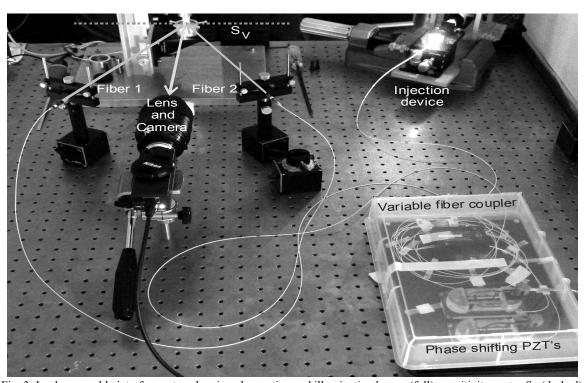
$\label{eq:speckle} Fig.~3: In plane speckle interferometer, showing observation and illumination beams (full), sensitivity vector <math>S_V$  (dashed), variable fiber coupler, phase shifting and injection devices.
