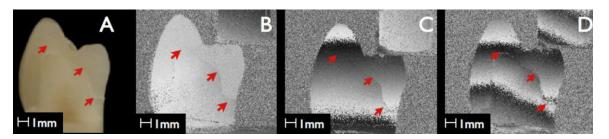
Fig. 3 – Prosthetic crown sample under different loads. (A) White light images. (B) Screenshot no. 08: force 36.78 N,  $\Delta F$ : 2.57 N (new ref: 41.01 N). (C) Screenshot no. 15: force 77.56 N,  $\Delta F$ : 5.29 N (new ref: 82.85 N). (D) Screenshot no. 33: force 64.09 N,  $\Delta F$ : 18.76 N (new ref: 41.01 N).
