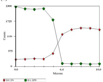
Fig. 7 – Results of elemental analysis across the feldspathic ceramic/zirconia interface by tracking the presence of Zr and Si, using the sectioned specimen. SEM image (a) with superposition of the line scan graph analysis (b).
