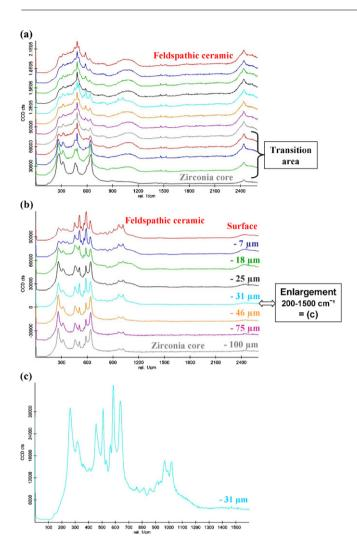
Fig. 3 – Raman line scans of the sectioned specimen (a) and in depth of thin-washed, unsectioned specimen (b). (c) represents an enlargement of the 31- $\mu$ m deep spectrum (from 200 to 1500 cm<sup>-1</sup>), identifying the main peaks of VM<sup>®</sup>9 and Y-TZP.
