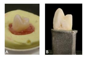
Fig. 25. The lost wax technique for the realization of the sample holder from a root imprint: A) print of roots in the wax, B) the chromium cobalt sample holder and the sample after a vertical cut.
