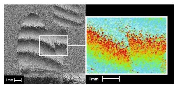
Fig. 8 – SI image sample "prosthetic crown" and displacements shown in a contour colored map. Behavior for a load of  $52.78 \, N$ ,  $\Delta F = 30.07 \, N$ , new ref:  $82.85 \, N$ .
