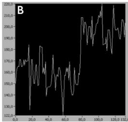
Fig. 6 – Prosthetic crown behavior at a load of 76.34 N,  $\Delta F = 6.51$  N, new ref: 82.85 N. (A) SI image: a single black line corresponds to the region of interest (ROI) used for displacement calculation. (B) Displacement curve along the black line, displacements in nm versus position in pixels. Step is about 43 nm.
