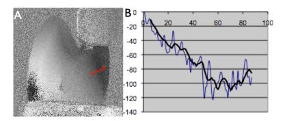
Fig. 48. Screenshot 2: Natural tooth behavior at a load of 39.21 N,  $\Delta F = 1.18$  N, N ref: 40.39 N. A) SI
