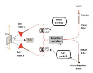
Fig. 16. SI set-up diagram.
