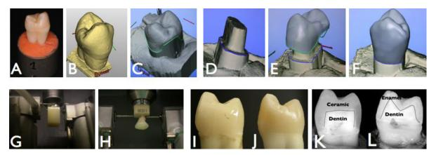
Fig. 1 – Cloning process: the intact natural crown sample (A), optical print (B), shaping (C), optical print of the second tooth prepared to receive the prosthetic clone (D), adaptation of the shaping on the tooth prepared (E), CAD finished, CAM ready (F), ceramic block in the milling unit (G), the prosthetic clone milled (H), the prosthetic clone cemented on the tooth prepared (I), the natural tooth (J), vertical cuts (K), prosthetic clone (L) natural tooth.
