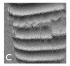
**Fig. 13**. Example for speckle images on a plaster model: A) white light image; B) reference speckle image; C) speckle image model under load in which the fringes correspond to the deformation of the plaster model.
