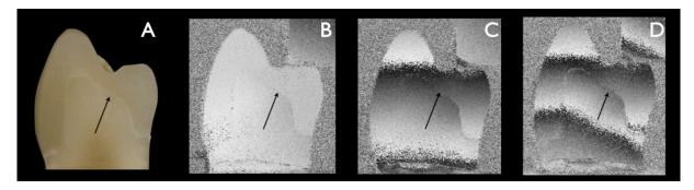
**Fig. 46.** White light and SI images for prosthetic crown sample; A) White light images; B) Screenshot N° 08: Force 36.78 N,  $\Delta F$ : 2.57 N (New ref: 41.01 N); C) Screenshot N° 15: Force 77.56 N,  $\Delta F$ : 5.29 N (New ref: 82.85 N); D) Screenshot N° 33: Force 64.09 N,  $\Delta F$ : 18.7 6N (New ref: 41.01 N).
