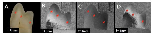
Fig. 2 – Natural tooth sample under different loads. (A) White light images. (B) Screenshot no. 04: force: 35.5 N,  $\Delta F$ : 35.5 N (new ref: 0). (C) Screenshot no. 13: force: 40.23 N,  $\Delta F$ : 0.16 N (new ref: 40.39). (D) Screenshot no. 24: force: 82.54 N,  $\Delta F$ : 13.96 N (new ref: 96.5).
