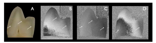
**Fig. 45.** White light and SI images for natural tooth sample; A)White light image, B) Screenshot N° 04: Force: 35.5 N,  $\Delta$ F: 35.5 N (New ref: 0); C) Screenshot N° 13: Force: 40.39 N,  $\Delta$ F: 0.16 N (New ref: 40.23); D) Screenshot N° 24: Force: 82.54 N,  $\Delta$ F: 13.96 N (New ref: 96.5).
