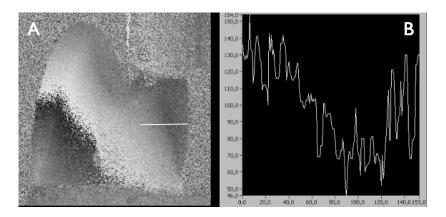
Fig. 47. Screenshot 1: Natural tooth behavior at a load of 38.65 N,  $\Delta F = 1.74$  N, N ref: 40.39 N. A) SI image: the single white line corresponds to the region of interest (ROI) used for the calculation of displacement. B) displacement curve along the white line. Displacements are shown in nm versus the position in pixels.
