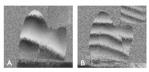
Fig. 52. Natural tooth (A) and prosthetic sample (B) under the same load (53.7 N)
