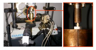
Fig. 42. Mechanical testing system and specimen between jaws.
