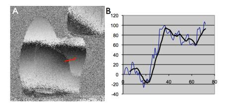
**Fig. 50.** *Screenshot 4:* **Prosthetic** crown behavior under a load of 72.85 N,  $\Delta F = 10$  N, N ref: 82.85 N. A) SI image: six red equal parallel lines are defined across the DEJ. B) Displacement curves: The blue curve represents displacement values along one of the six red lines. The black curve is the mean value fitting of the 6 blue curves. The displacement was approximately 95 nm.
