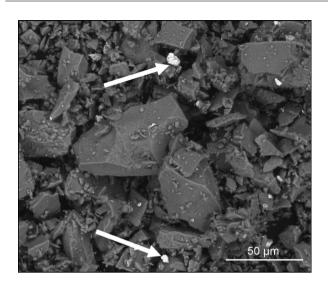
Fig. 6 – SEM observation of the powdered feldspathic ceramic (VM<sup>®</sup>9). White crystals (white arrows) correspond to zirconia crystals.
