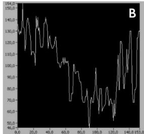
Fig. 4 – Natural tooth behavior at a load of 38.65 N,  $\Delta F = 1.74$  N, new ref: 40.39 N. (A) SI image: the single white line corresponds to the region of interest (ROI) used for the calculation of displacement. (B) Displacement curve along the white line, displacements in nm versus position in pixels. Step is about 43 nm.
