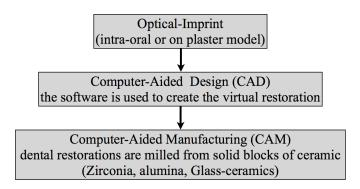
Fig. 1. The general principles of CAD/CAM in prosthetics
