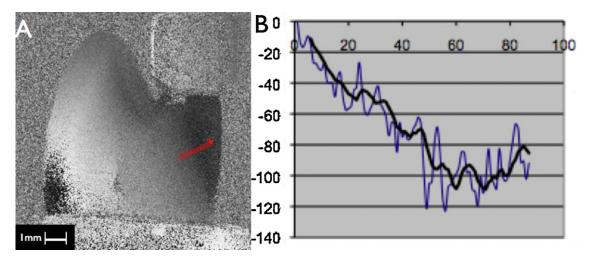
Fig. 5 – Natural tooth behavior at a load of 39.21 N,  $\Delta F = 1.18$  N, new ref: 40.39 N. (A) SI image: six red equal parallel lines, 1 pixel separated, are defined across the DEJ. (B) Displacement curves: blue curve: displacement values along one of the six red lines. Black bold curve is the mean value fitting of the 6 blue curves. (For interpretation of the references to color in this figure legend, the reader is referred to the web version of the article.)
