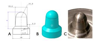
**Fig. 11.** A shape made by CAD/CAM can be perfectly calibrated and reproduced. A) the projection, B) the 3D shape design, C) the machined shape.
