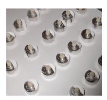
Fig. 41. Specimen preparation: the superstructures (ceramic caps) are adhesively glued on the aluminum-milled infrastructure.
