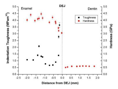
**Fig. 7.** Typical profiles of the Vickers hardness and indentation toughness taken normal to, and across, the DEJ from the enamel to the dentin in a human molar (34).
