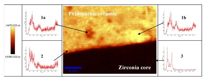
Fig. 4 – Raman microanalysis using the selection of the peaks of interest in the feldspathic ceramic. Spectra corresponding to different crystalline phases are presented in the lateral columns: Feldspathic ceramic (1a = glass matrix, 1b = crystalline phase), interdiffusion area (2), zirconia core (3).
