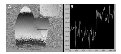
**Fig. 49.** *Screenshot 3:* Prosthetic crown behavior at a load of 76.34 N,  $\Delta F = 6.51$  N, N ref: 82.85 N. A) SI image: a single black line corresponds to the region of interest (ROI) used for the displacement calculation. B) The displacement curve along the white line; in this case, the step was approximately 43 nm.
