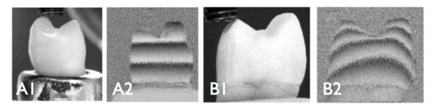
**Fig. 43.** Whole samples under loading: A) natural whole tooth, B) prosthetic clone under white light and speckle picture under loading. The fringes show the movement of the crowns under a load. The root and the sample holder were stable, and only the enamel cap and the ceramic cap were moving. There is no fringe on the sample holder (A2) and at the beginning of the roots (B2).
