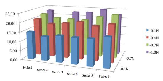
**Fig. 55.** Responses to stress exhibited by the samples; the evolution of apparent stiffness (kN/mm) for different loading force levels was calculated.
