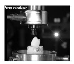
Fig. 27. Sample powdered (whole tooth) in place before loading.
