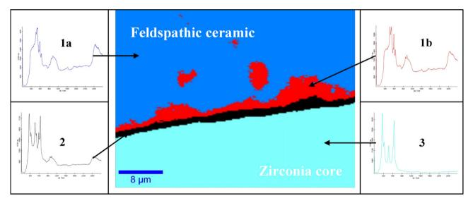
Fig. 5 – Raman microanalysis of the feldspathic ceramic/zirconia interface using K-Means Cluster Analysis function. Representative spectra from the four specific regions are presented in the lateral columns: Feldspathic ceramic (1a = glass matrix, 1b = crystalline phase), interdiffusion area (2), zirconia core (3).
