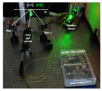
**Fig. 17.** This figure shows the plane speckle interferometer with the observation and illumination beams (solid lines), sensitivity vector Sv (dashed line), variable fiber coupler, and the phase shifting and injection devices.
