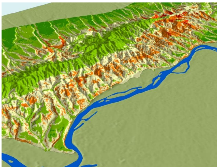
Figure 8. A 3D view from the northeast, with the Danube riverside (vertical exaggeration 2.7) susceptibility map legend: green – low, yellow – medium, red - high
