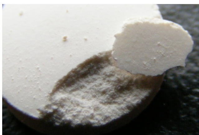
Fig. 3 Tablet capping (S0)
