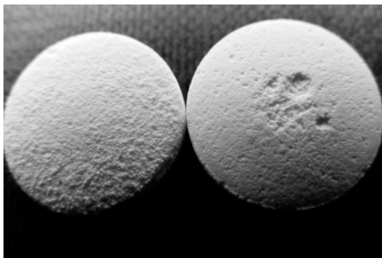
Fig. 4 Surface of S4 (left) and S5 tablets (right) after 20 min disintegration at pH 3.0
