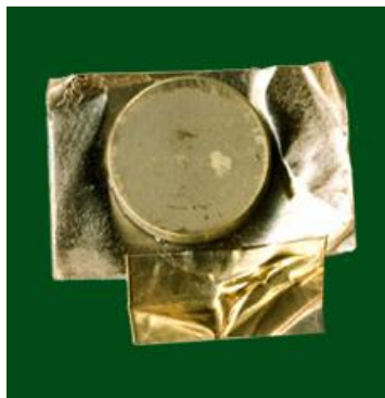
Figure 24A. Macroscopic picture of a Ti disc treated with 1% NaF at pH 4.5 and incubated with S. mutans for 5 days. The bacterial cells cover almost the whole surface.
