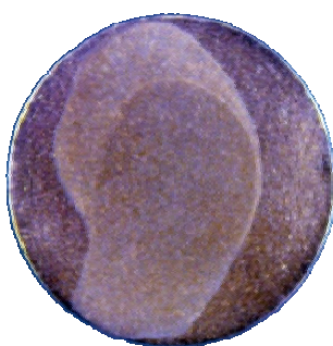
Figure 12. Macroscopic image of a disc smeared with the gel (12 500 ppm F^- and pH 4.8) revealing the macroscopic surface change caused by the high concentration of F^- .
