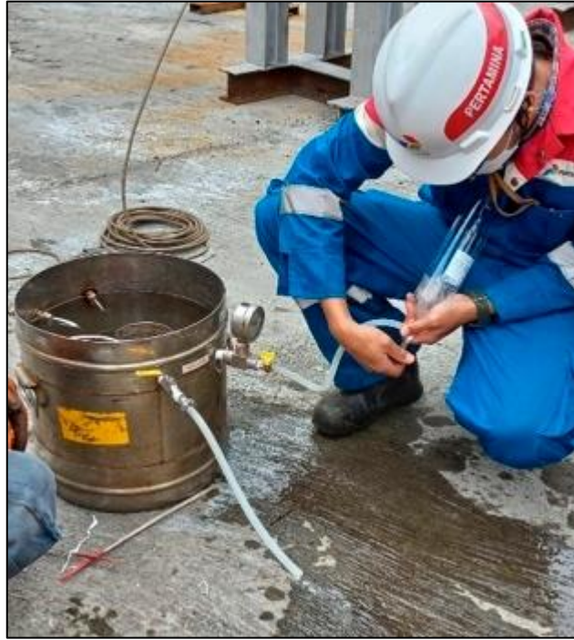
Figure 24. Gas sampling collection
