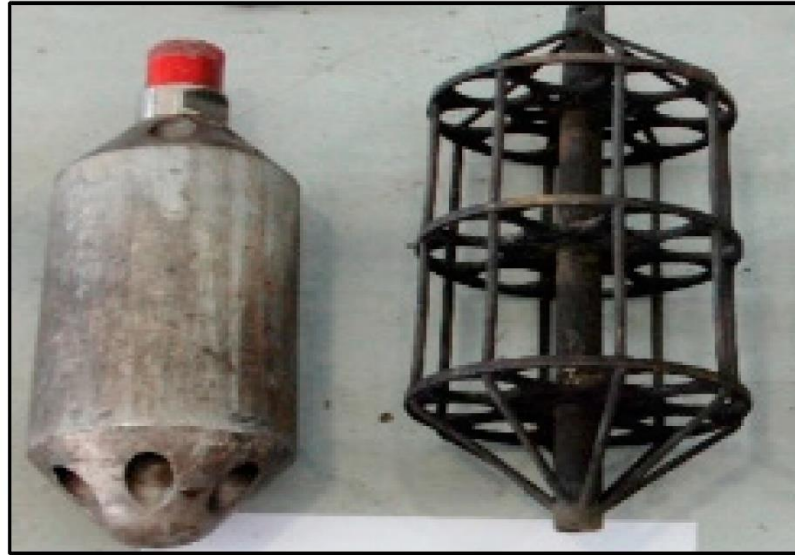
Figure 27. Well integrity assessment using go-devil.
