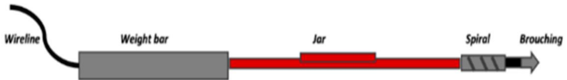
Figure 34. Broaching surface tools.
