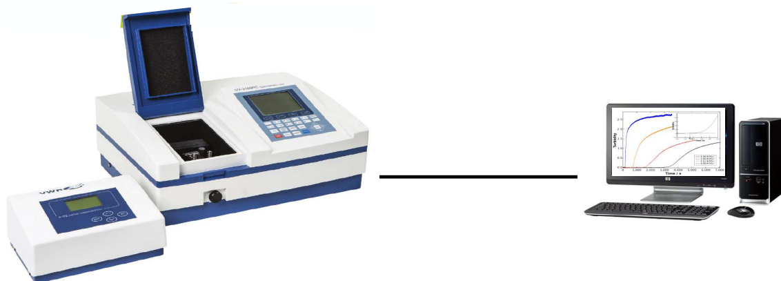
Figure 4.1: Experimental setup for the measurement of turbidity of a well-stirred solution
