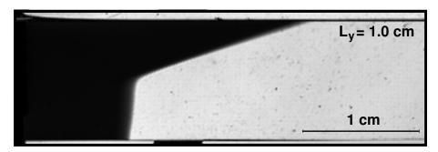
Figure 6. The recorded image of the reaction front during the sounding rocket experiment in the 10 mm wide cell.
