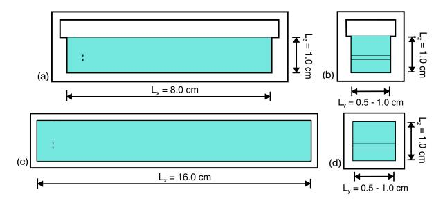
Figure 1. The geometry and dimensions of the cells used during the parabolic flight experiment. The cross section of the cell with the possibility of creation free liquid-gas interface in the *xz*-plane (a), in the *yz*-plane (b), the cross section of the fully filled cells in the *xz*-plane (c) and in the *yz*-plane (d).
