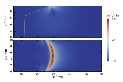
Figure 8. The velocity flow field and the front shape (yellow line) in the xz-plane along the centerline of the cell (top) and in the xy-plane of the fluid-gas interface (bottom) as a result of the fluid dynamic calculations.
