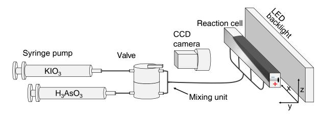
Figure 2. Schematic diagram of the experimental setup used for the parabolic flights.
