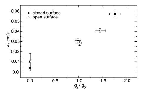
Figure 4. Velocity of front propagation as a function of gravitational acceleration for various cell types.
