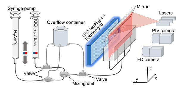
Figure 3. Schematic figure of the setup used for the sounding rocket experiment.
