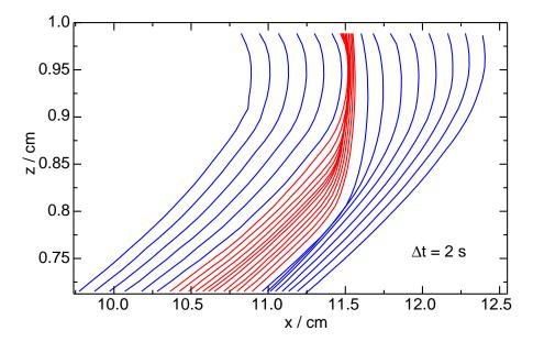
Figure 5. Spatiotemporal evolution of front profiles with  $\Delta t = 2$  s for a reaction front propagating left to right in the absence of liquid-air interface. The blue lines represent the front shapes recorded in hypergravity phases while the red lines the shapes in microgravity.
